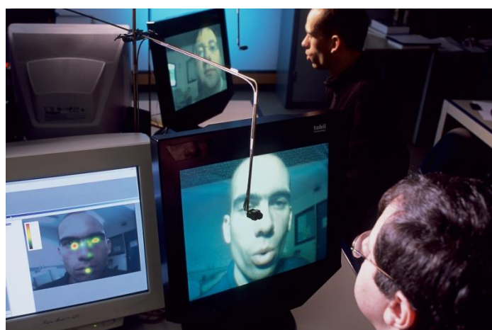
Figure 1. First experimental setting used by Bailly et al (G. Bailly, Raidt, & Elisei, 2010) to study mutual gaze patterns using computer-mediated face-to-face interactions.
