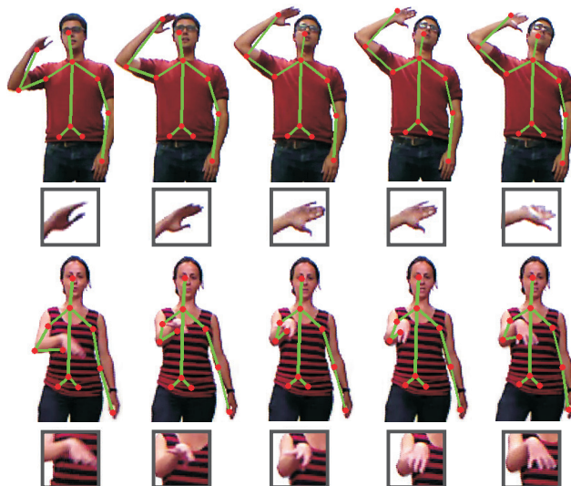
Figure 1. Examples of two-scale gesture decomposition: upper body movement and hand articulation. The gesture in the top row can be fully characterized by large-scale body motion, whereas in the one below, subtle finger movements play the primary role.
