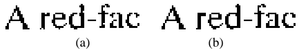
Figure 3. An example binarized with Sauvola's method (a) with the MRF method (b)
