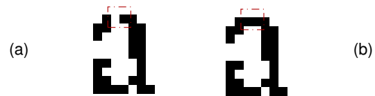
Fig. 6. Low resolution example binarized with Sauvola's method (a) with the MRF method (b)
