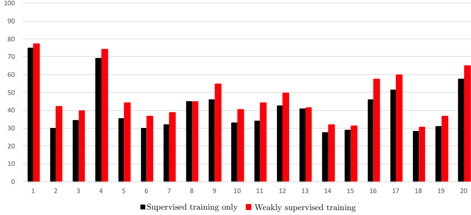
Figure 64 – Average segmentation accuracy per class obtained with the supervised method (in black) and after the weakly supervised adaptation of the segmentation learner f_s(\theta_s) to the real data (in red). These results were obtained using 100 manually labeled images from the NYU Hand Pose Dataset [296] (NYU-100). The horizontal axis shows numbers of hand segments (see Figure 63).
